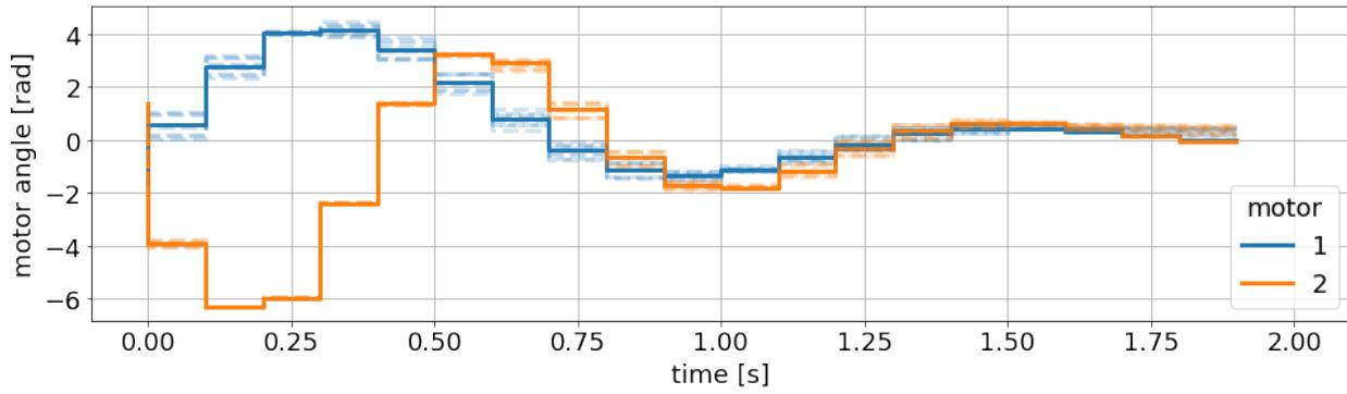
The simulated trajectory with the nominal value of the parameters follows almost exactly the nominal open-loop predictions. The simulated trajectory is bounded from above and below by further uncertain scenarios.
