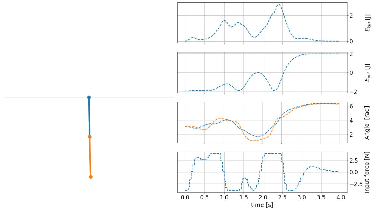
The open-loop prediction looks perfectly fine! We see that within the horizon the potential energy settles on a plateau greater than zero, while the kinetic energy becomes zero. This indicates our desired up-up position. Both angles seem to reach  $2\pi$ .
