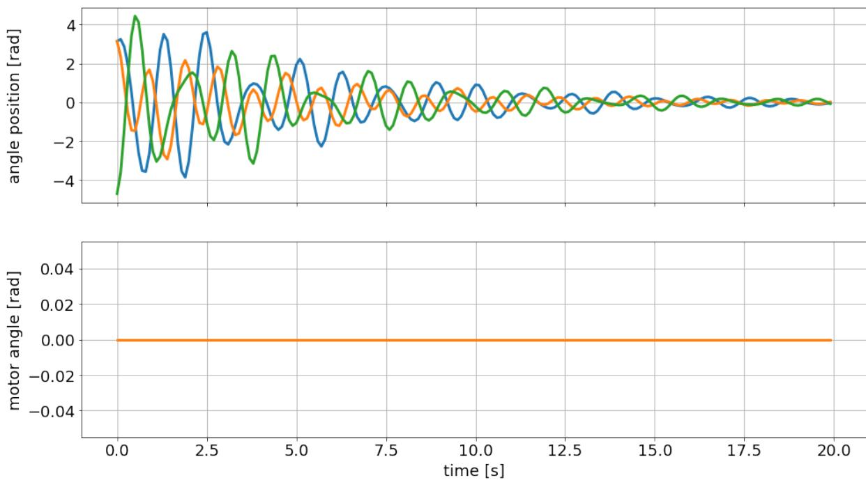
As desired, the motor angle (input) is constant at zero and the oscillating masses slowly come to a rest. Our control goal is to significantly shorten the time until the discs are stationary.
