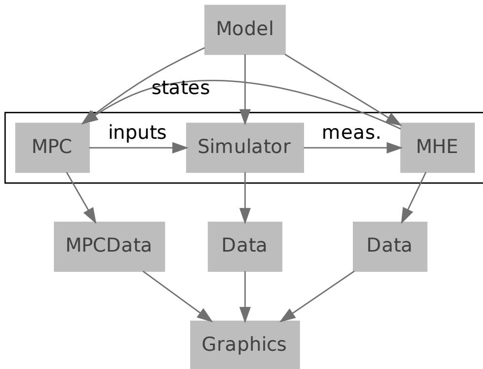
Fig. 4: **do-mpc** control loop and interconnection of classes.
