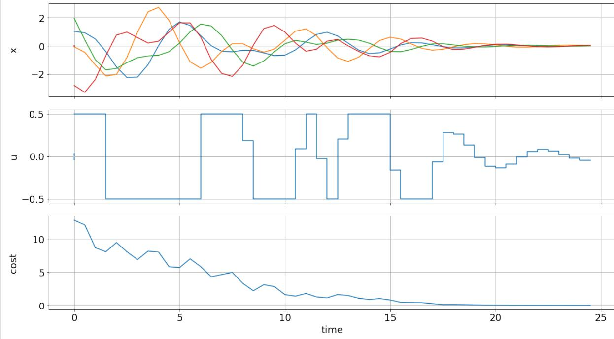
We can see that the control objective was successfully fulfilled and that bounds, e.g. for the control inputs are satisfied.
