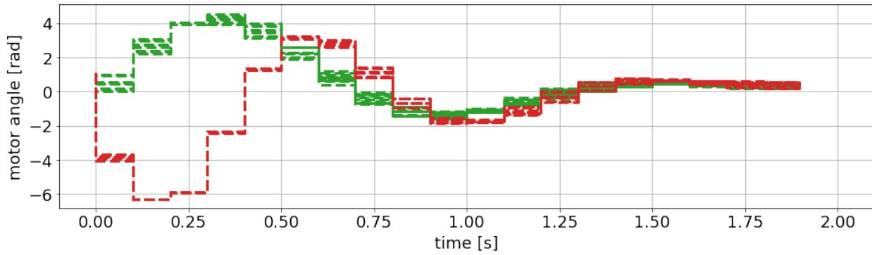
We are seeing the predicted trajectories for the states and the optimal control inputs. Note that we are seeing different scenarios for the configured uncertain inertia of the three masses.
